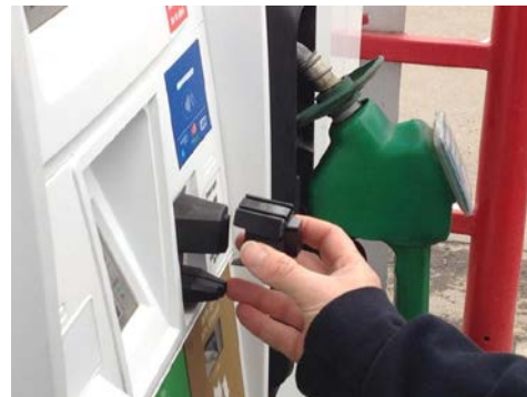
Gas pump skimming device
